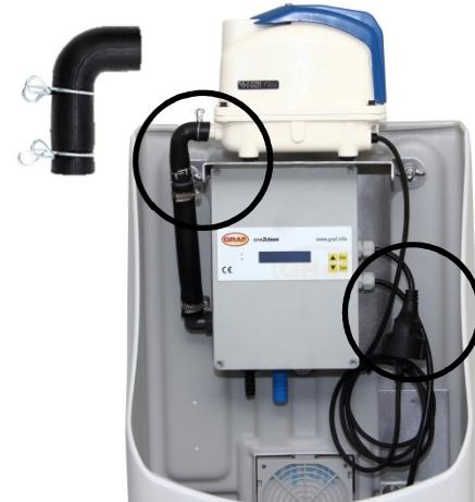
The compressor is placed on top of the control unit. Use the rubber bracket for the air connection. For the power connection, the compressor's connector is plugged into the socket on the control unit.
