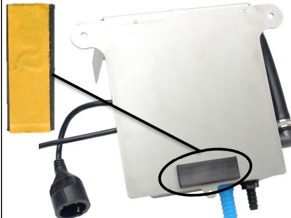
Before installing the control unit, a strip of foam rubber must be glued to the back of the control unit.
