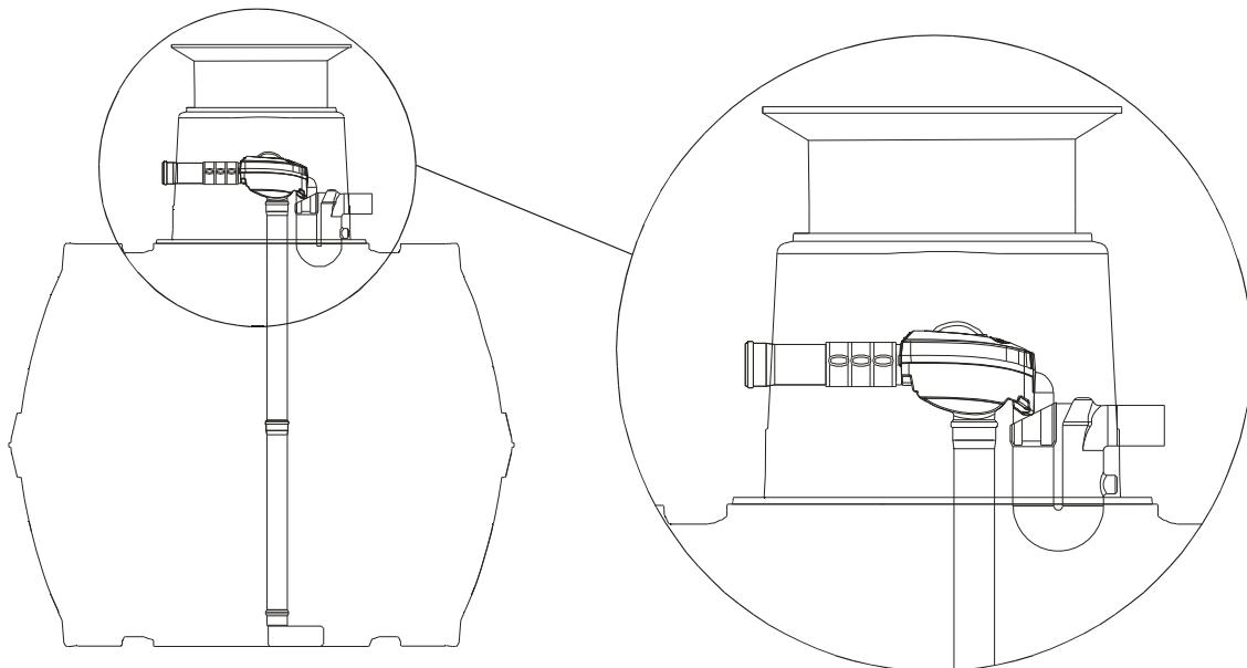
Insert the filter, prepared with the inflow pot (calmed down), in the tank.
